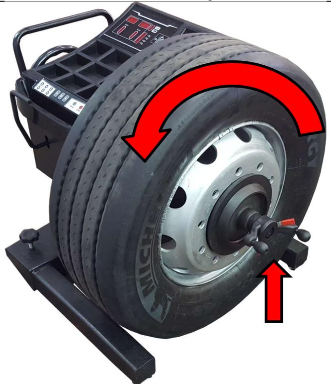
The balancing unit and the wheel can then be lifted. This should be about 2 cm above the ground.
