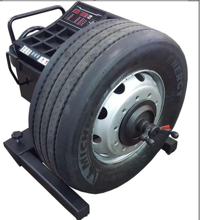
If the rim is not precisely centred on the shaft, the height can be adjusted by turning the handwheel.
