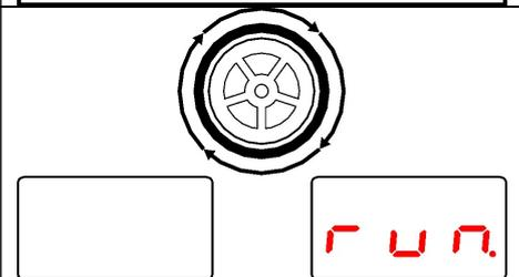
The display shown opposite appears after the balancing process. The braking process can now be initiated. Attach the calibration weight (200 g) to the inside of the wheel rim.
